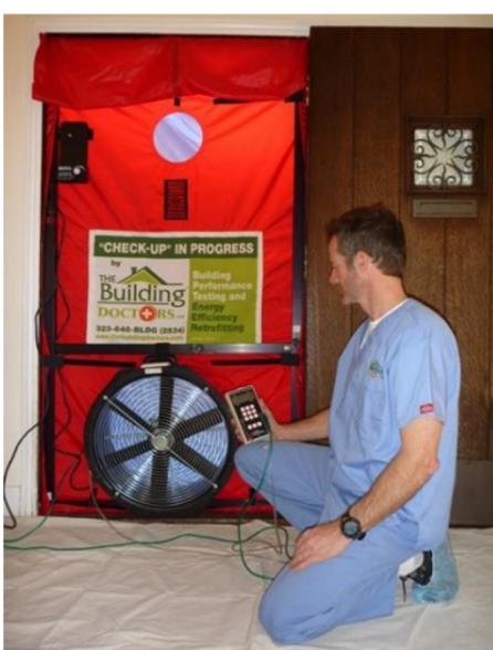
Testing the residence for air leakage is part of the Weatherization home energy audit.
